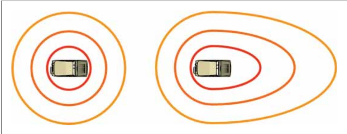
Figure 5: Modified cost field to dissuade AGV from planning to drive in front of other vehicles
