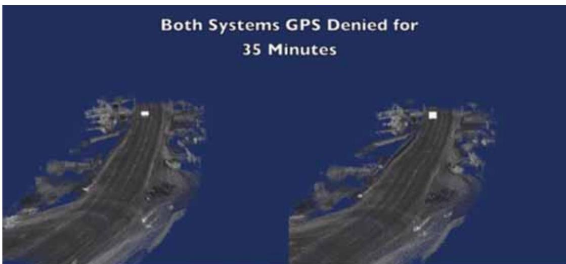
Figure 4: Integration of Candidate 1 (Left) and Candidate 2 (Right) sub-system into Multi-frame Autonomous Navigation Architecture provides GPS denied operation of LiDAR registration system over 40 times longer, and at one tenth the cost, of baseline INS system
