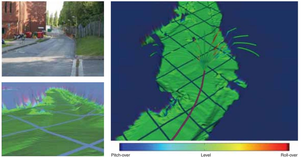
Figure 2: NURBS–KF modelling of surface geometry. Top left – Visual viewpoint of scene to be modelled. Bottom left – A NURBS–KF surface generated from Velodyne HDL-64 data captured from the same area. Right – Trajectories evaluated across the surface to determine potential pitch-over and roll-over conditions
